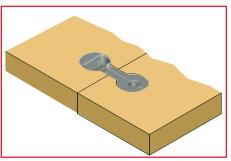
2 FASTEN THE QUICK BY USING A S6mm ALLEN WRENCH OR CORDLESS DRIVER-DRILL WITH S6mm HEXAGONAL BIT.
