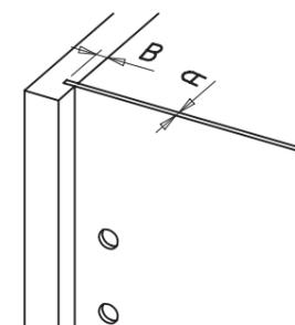
Presence and thickness of the back panel (A), depth of the milling (B).
