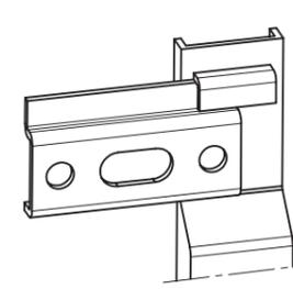
If the bracket is only partially hooked onto the wall plate.
