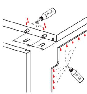
Presence, position and quantity of dowels, connection fittings and glue.
