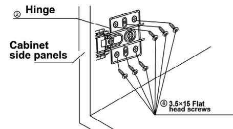
Caution! If it is not possible to open the cabinet door completely. You may need to add padding or Z-shaped between the cabinet side panels and the hinges
