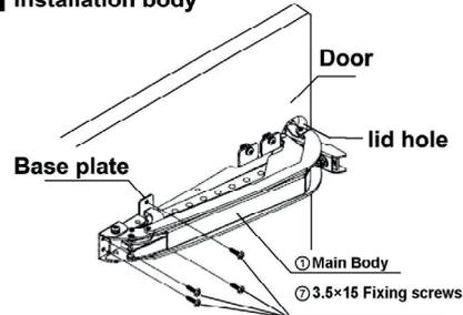
⚠ Make the hinge base plate flat against the door plate, adjust the screw in the center position
